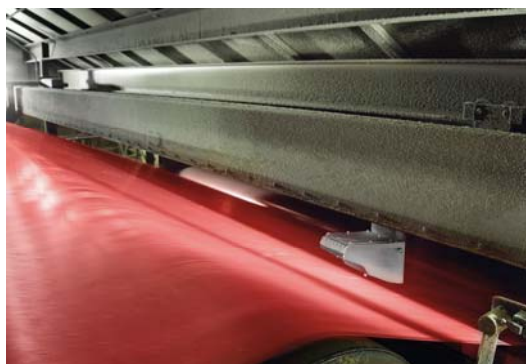
Fastpap ComboSprint rengör viran under drift.
